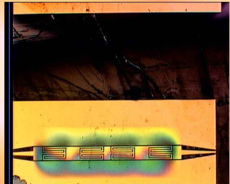
GaAs membrane supported double folded open end series stub band pass filter structure for 38 GHz
